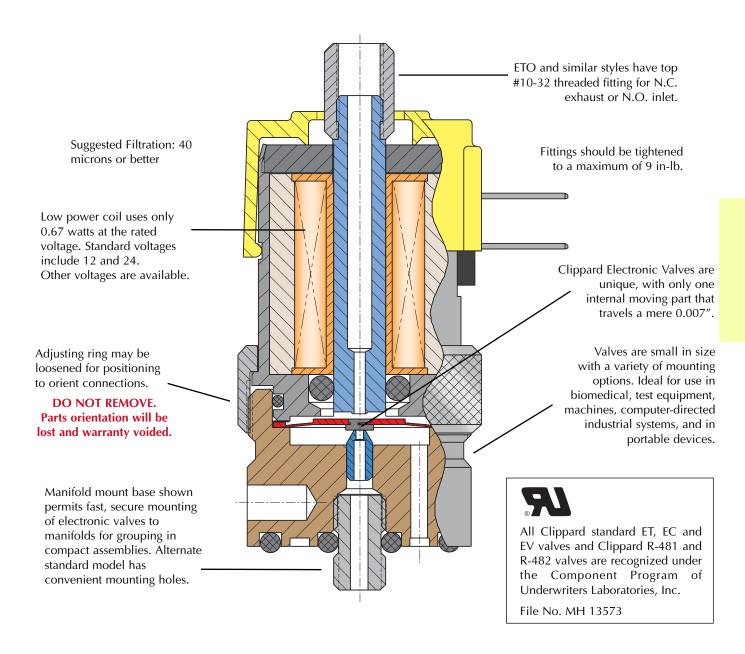
Clippard Minimatic electronic valves are precision-built 2-way or 3-way control valves, utilizing a unique, patented, valving principle. There are no sliding parts. Complete poppet travel is a mere 0.007". As a result, low power consumption and exceptionally long life are major benefits of this design.
